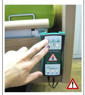
For *Mobility Monitor* to be able to detect movements correctly, the system must be adjusted/calibrated to the bed and the mattress. First unlock the keys
