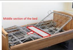
Remove the mattress. Check, which is the non-movable middle section of the bed (at pelvic level).
