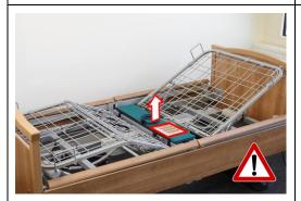
Using the straps attach the sensor unit to the non-movable middle section of the bed.
