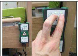
Attach the control unit to the bed and connect the sensor unit cable. Now connect the device to the power supply. Connecting to the nurse-call system is optional.
