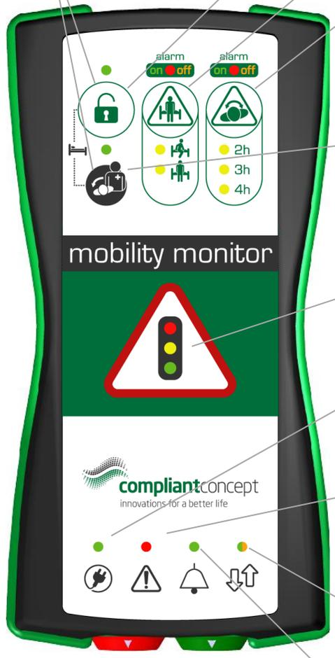
The diagram shows the Mobility Monitor device with four main sections: **Zone de commande** (Control Zone), **Zone d'affichage** (Display Zone), **Zone de status** (Status Zone), and **Connexions** (Connections). Each section contains specific controls and indicators described in the callouts.
